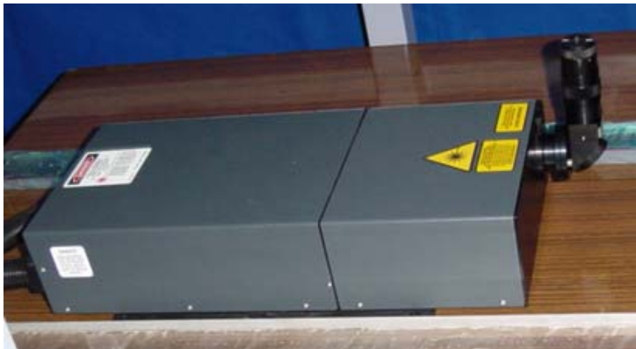
Figure 3.6. A Nd.YAG Laser Source
